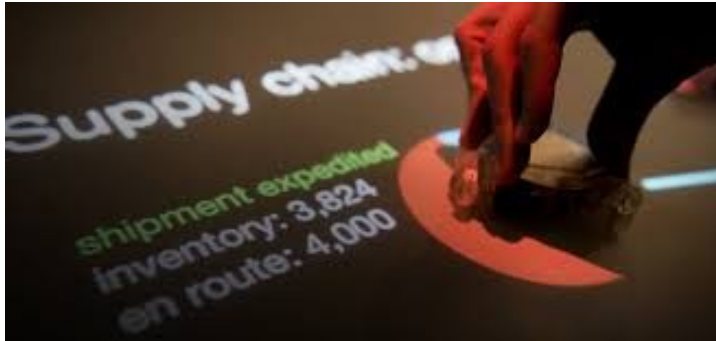
Figure 3.2 The Thumbles combine the advantages of a GUI with the intuitiveness that a physical object implies
