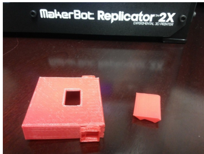
Figure 4.4 Our car parts (platform and bumper) after printing
