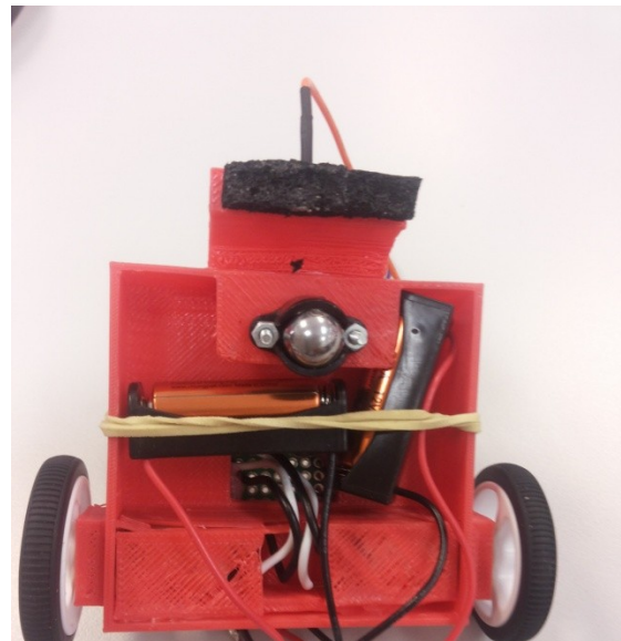
Figure 5.1 View of our car from below. We can observe the presence of the two batteries and the 'free wheel' that replaces two conventional front ones.
