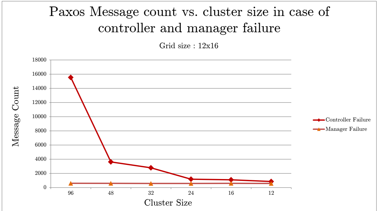
Figure 8.11: Message count vs. cluster size in 16 \times 12 grid
