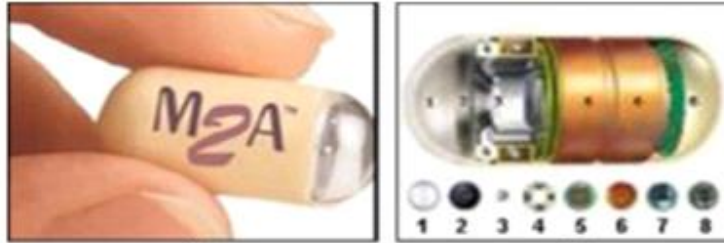
Figure 1.13. M2A Capsule and schematic diagram of its components
