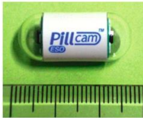
Figure 1.15. PillCam ESO (11x26MM); capsule endoscope for investigating esophageal diseases
