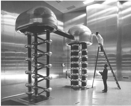
Figure 2.1: The Cockcroft-Walton accelerator [6].
