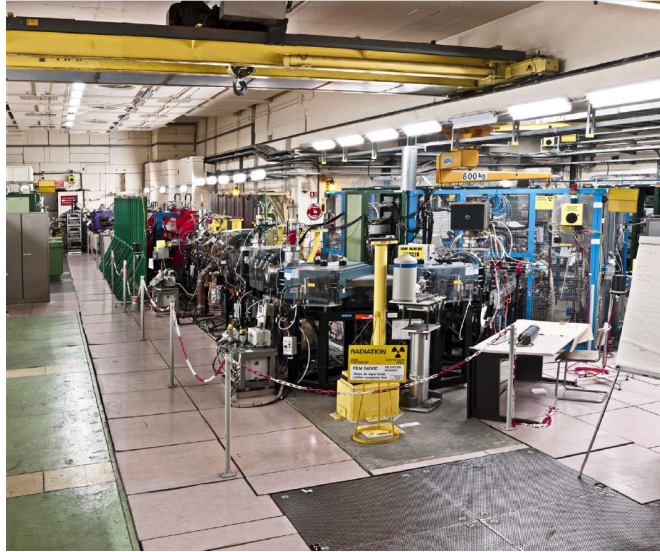
Figure 4.2: The Linac3 Layout. At the right part of the picture is the source in the cage and the spectrometer. At the foreground, the LEPT, the RFQ, the MEPT and the IH tanks of the structures can be recognized. [47]
