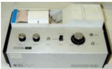
im8. The Cambridge VS4, a popular ECG instrument of the 1970's and 1980's. Solid state technology [2]
