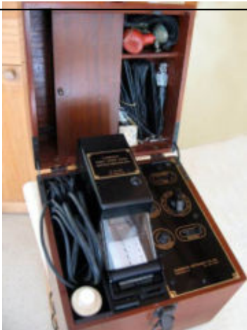
im7. The Cambridge Simpliscribe, a popular ECG instrument of the 1950's and 1960's. Vacuum tube technology [2]
