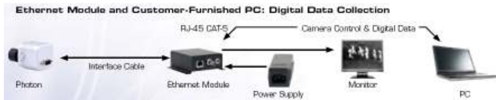
Figure 4. 11 Configuration of the transmission system [Fli08].
