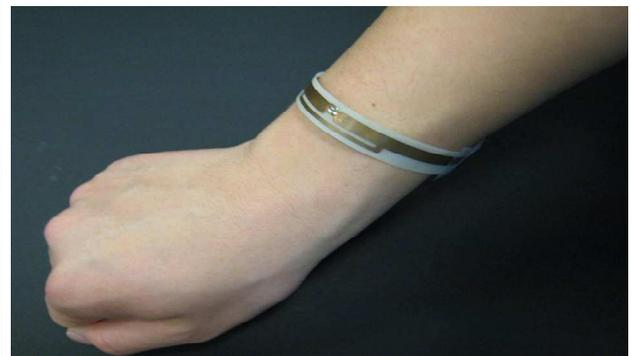
**Figure 4.4** Wearable RFID tag on wrist for medical monitoring
