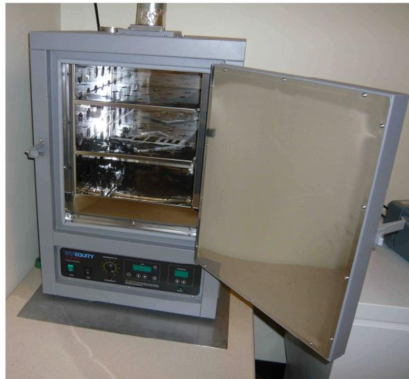
**Figure 4.20** Test Equity FS series industrial oven for performing curing of the prototype antenna
