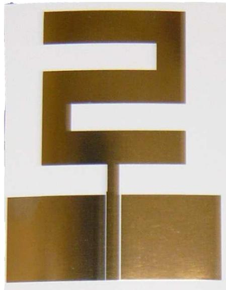
**Figure 4.17** Prototype of the conductive inkjet-printed antenna
