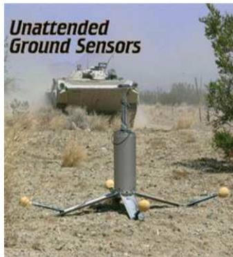
**Figure 2.3** Wireless Sensor Network Node
