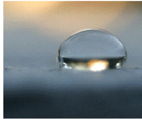
**Figure 4.2** Magnified droplet of water sitting on a paper substrate
