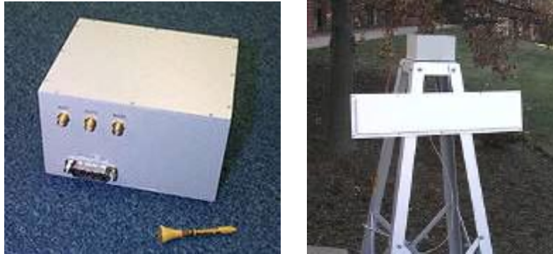
Figure 6.9: Hummingbird UWB Altimeter and Collision Avoidance Sensor.
