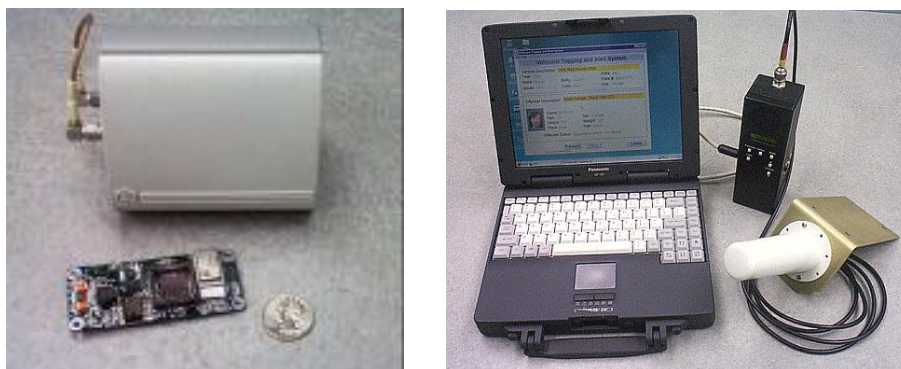
Figure 6.5: Ultra Wideband Tag & Tag Reader ( Vehicular Electronic Tagging and Alert System ).
