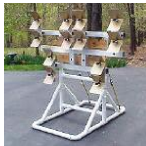
Figure 6.15: UWB Antenna Array ( Spider ) for Extended Range Intrusion Sensor.
