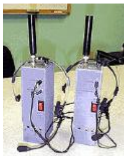
Figure 6.6: UWB Wireless Intercom Communications System (WICS).
