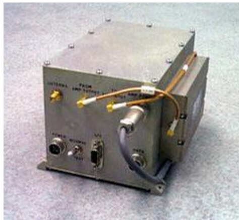
Figure 6.3: Asymmetric Video/Command & Control UWB Transceivers.
