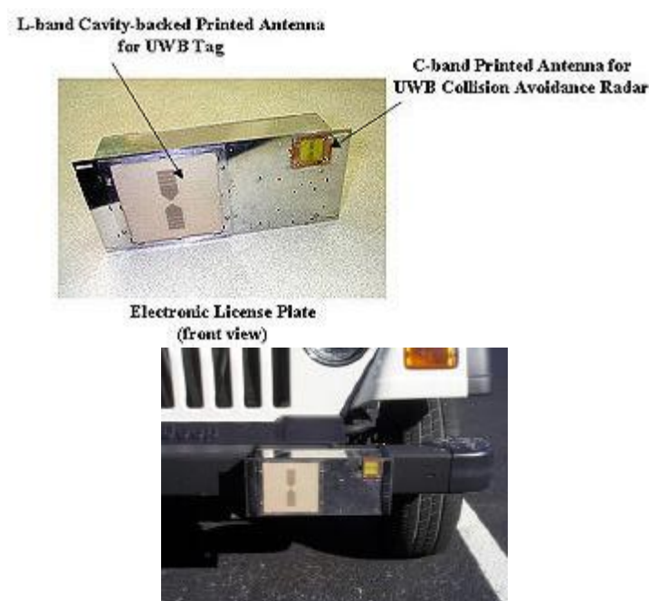
Figure 6.11 : UWB License Plate (Tag + Collision Avoidance Radar).
