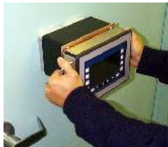
Figure 6.14: UWB Through-the-wall Intrusion Sensor.
