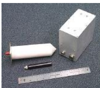
Figure 6.8: UWB Precision Geolocation System Transceiver.
