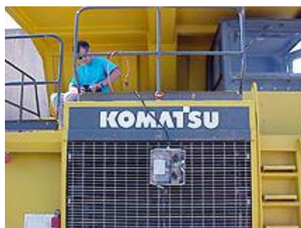
Figure 6.10: UWB Backup Sensor.
