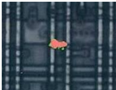
Figure 2.8. TDDB-induced leakage between adjacent wires of the same metal layer.
