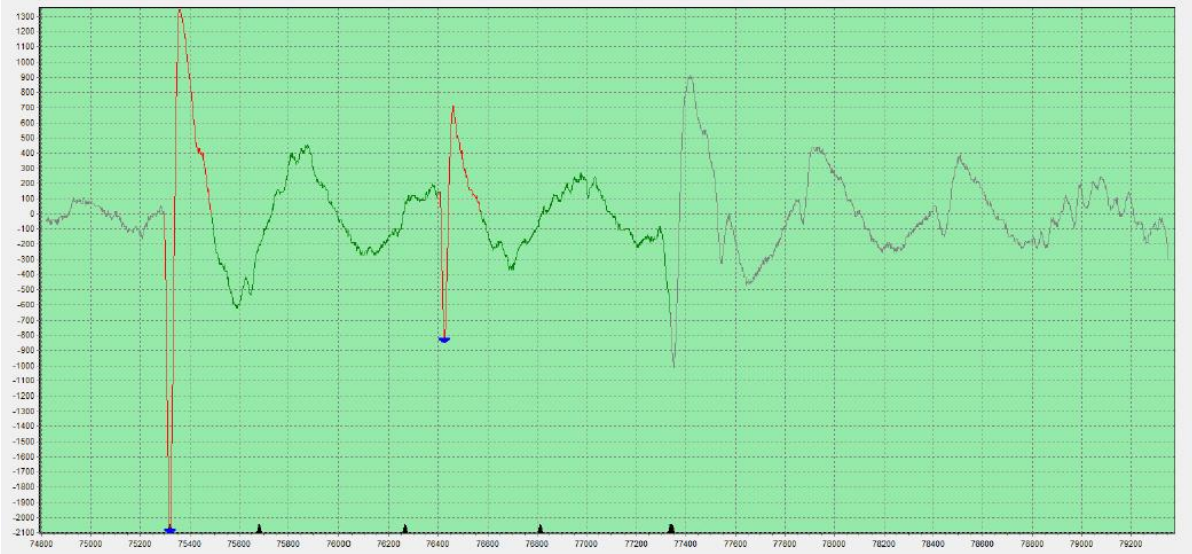
Figure 86: Phase L3(T) at 23 kV pulse with TDR method
