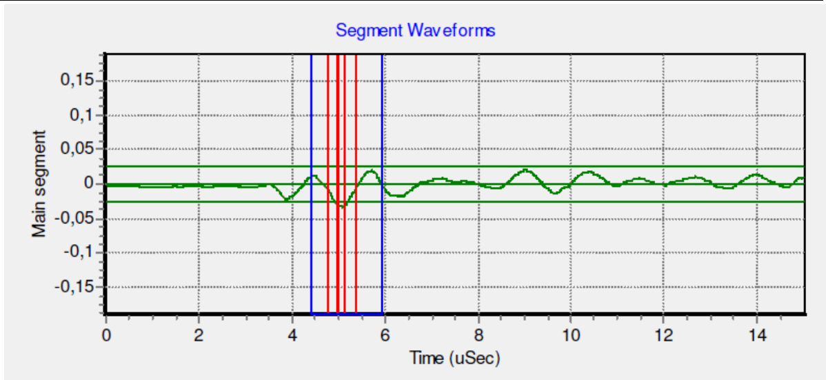
Figure 106: Form of one partial discharge pulse (14 \mu s)
