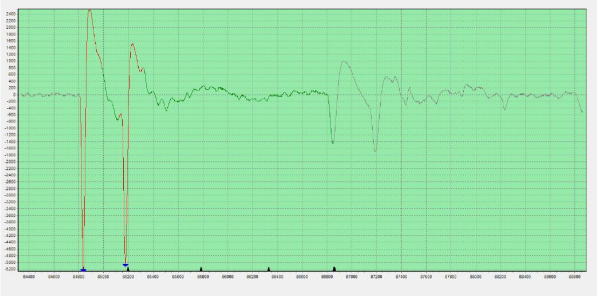
Figure 85: Phase L2(S) at 21 kV pulse with TDR method
