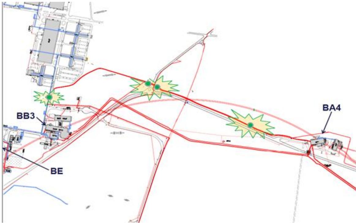
Figure 52: Location of intervention between BE and BA4 substations [Source: D. Bozzini TS/EL-HT, 10 November 2008, CERN]
