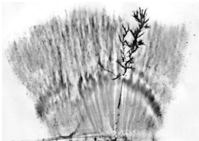
Figure 10: Electrical tree grown inside a water tree in laboratory conditions.
