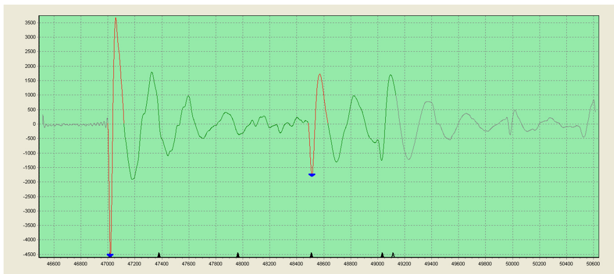
Figure 94: Phase L3(T) at 25 kV pulse with TDR method
