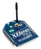
Fig 5.5 Digi XBee [XBee00]
