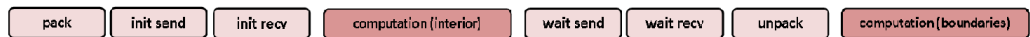
Figure 4.15: Overlapping implementation of heat equation with non-blocking communication: execution pattern for a single thread for each time step
