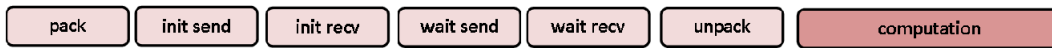
Figure 4.13: Non-overlapping implementation of heat equation: execution pattern for a single thread for each time step
