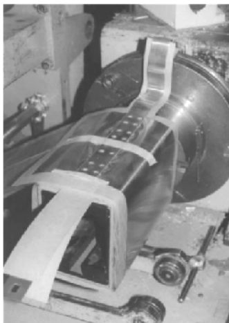
Spiral Sheet Low-voltage Winding
