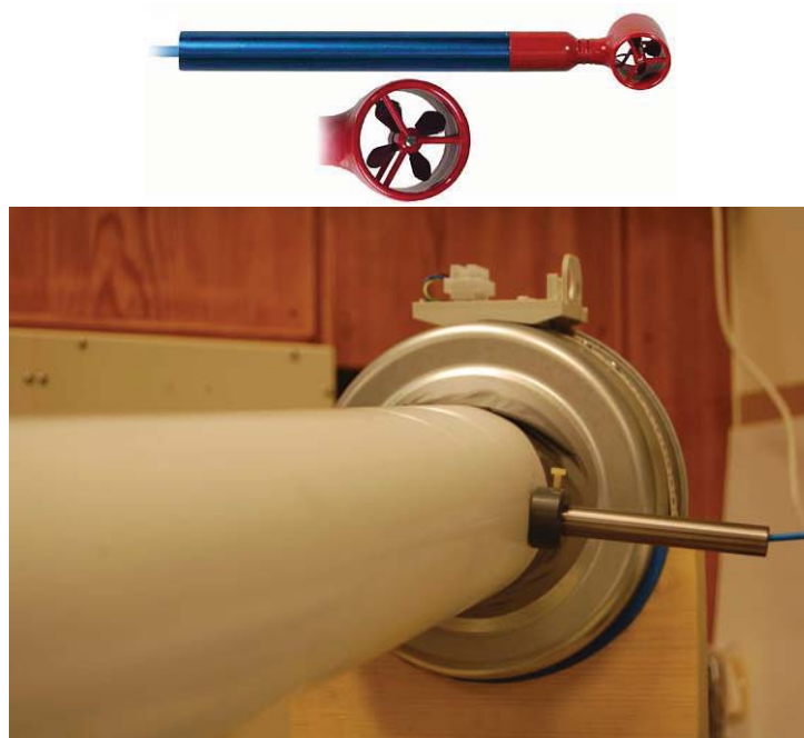
Figure 4.9: MiniAir64 mounted in the outlet pipe.
