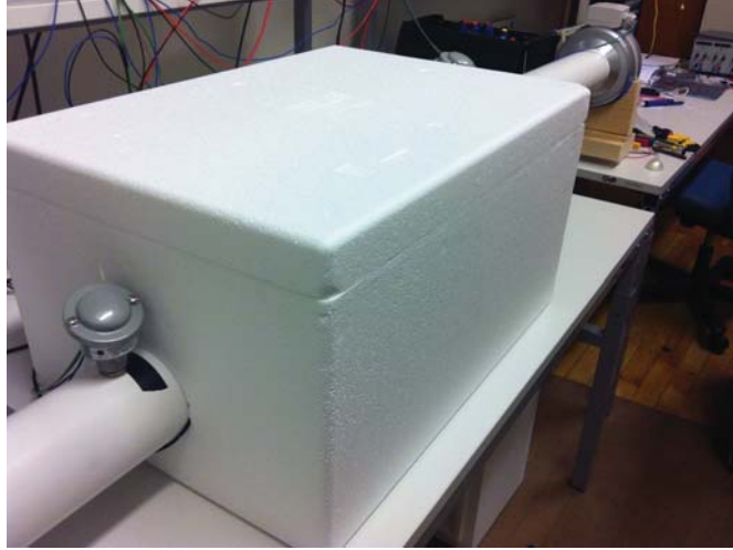
Figure 4.6: A 355mm x 265mm x 545mm chamber made by EPS used in this project
