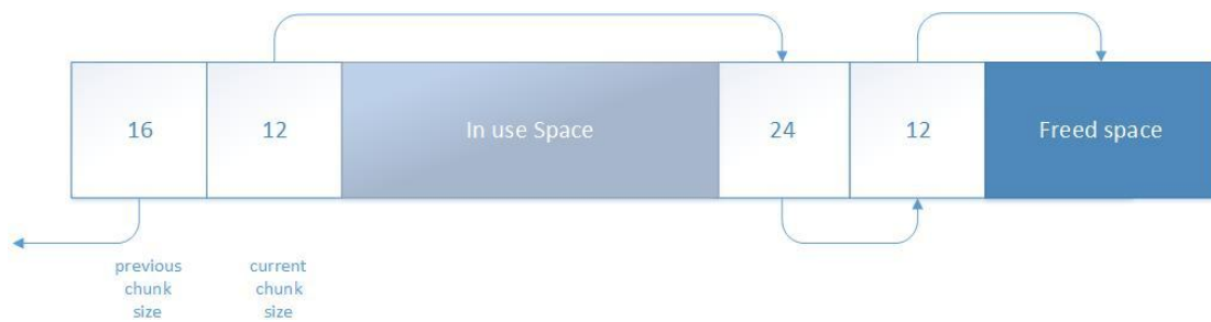
Figure 1-4: A fragment of a freelist-based heap, as used by Linux and Windows. Object headers precede each object, which make it easy to free and coalesce objects
