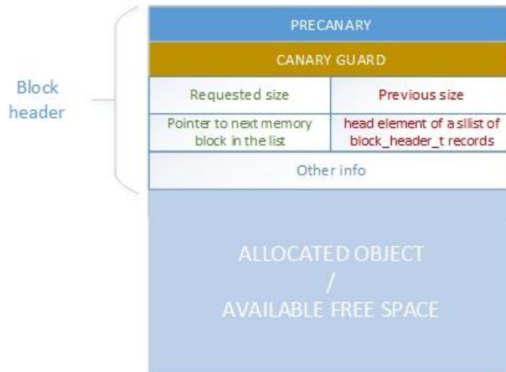
Figure 4-5: Block header fields used by canary mechanism in order to distinguish blocks' states. Red denotes the one used for free blocks while green the one used for in use blocks.
