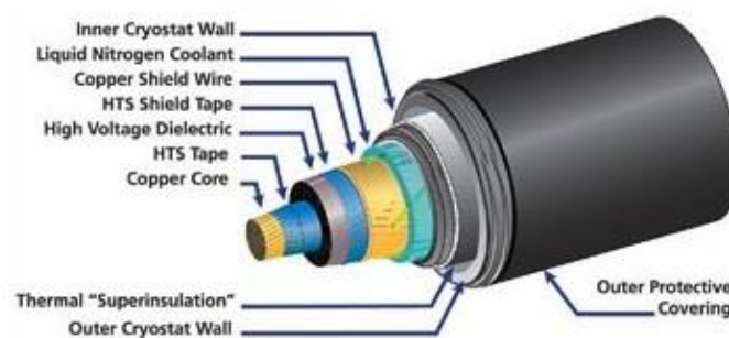
Example Superconductor cable design by Nexans
