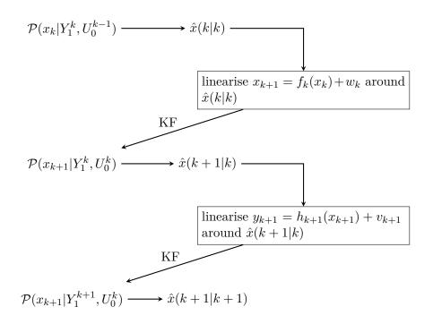
Figure 2.1: Extended Kalman Filter dynamic concept
