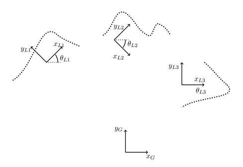
Figure 4.13: Landmarks and Local Frames
