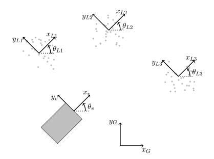
Figure 4.5: Map and Landmark Pose Frames
