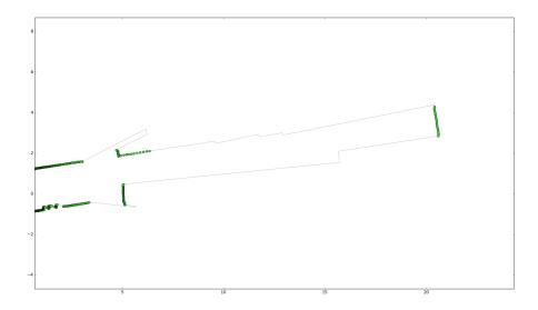
Figure 5.1: Scan segmented in candidate Landmarks
