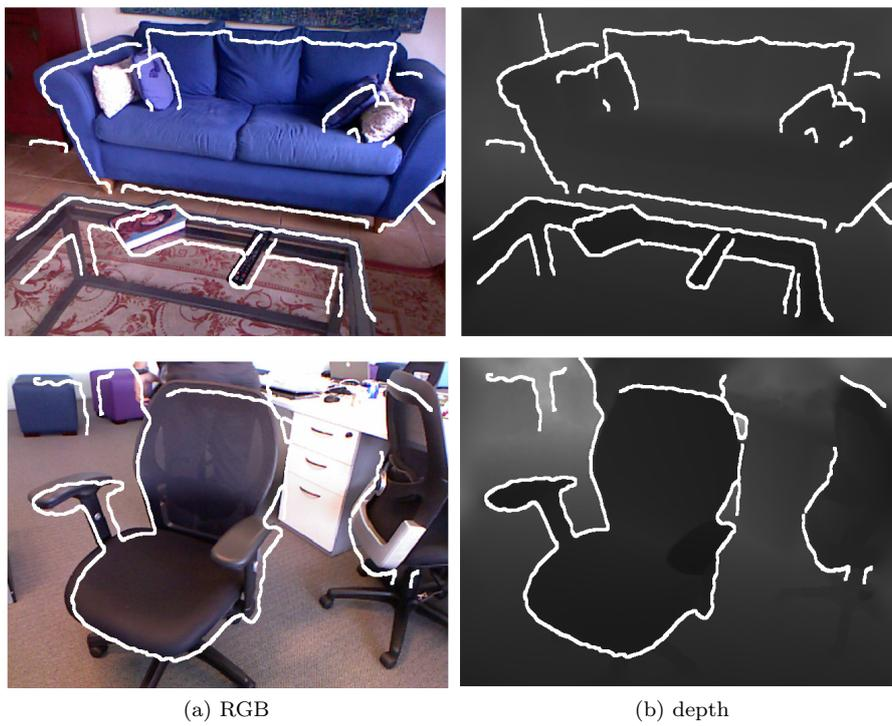
Figure 4.9: Two images with apparent misalignment between RGB and depth image. The white lines are the edges of the depth image and where they are represented in the RGB image.
