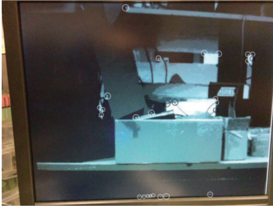
Figure 2.4: Harris Corner feature detected by their FPGA hardware method
