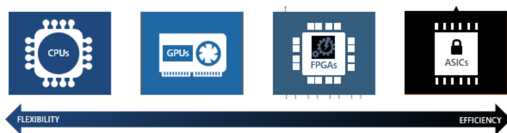
Figure 3.19: Flexibility vs Efficiency: CPU, GPU, FPGA, ASIC technologies.
