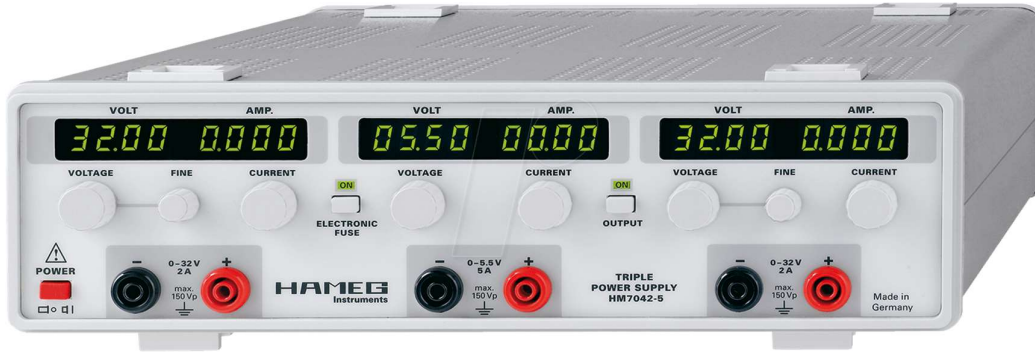
Figure 3.10. Hameg7042-5. Two of these power suppliers (totally five channels) used for the power supply of the whole setup.
