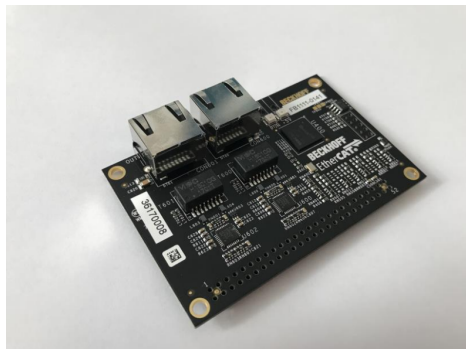
Figure 4.15: The EtherCAT slave ESC [17].
