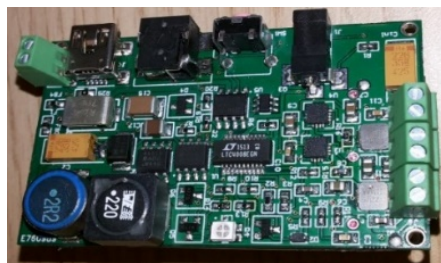
Figure 21. PCB of the power module sensor board.
