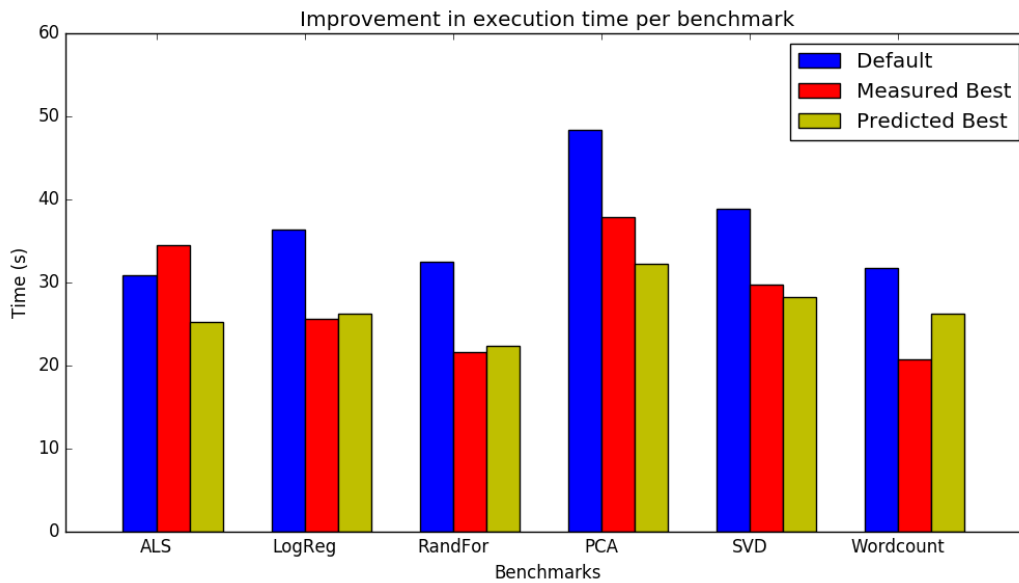
Figure 5.6: Comparing default, best measured and best predicted execution time for validating benchmarks and tiny size of input data
