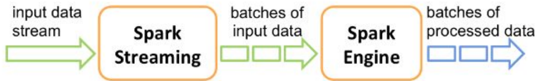
Fig. 9: Spark Streaming data flow
