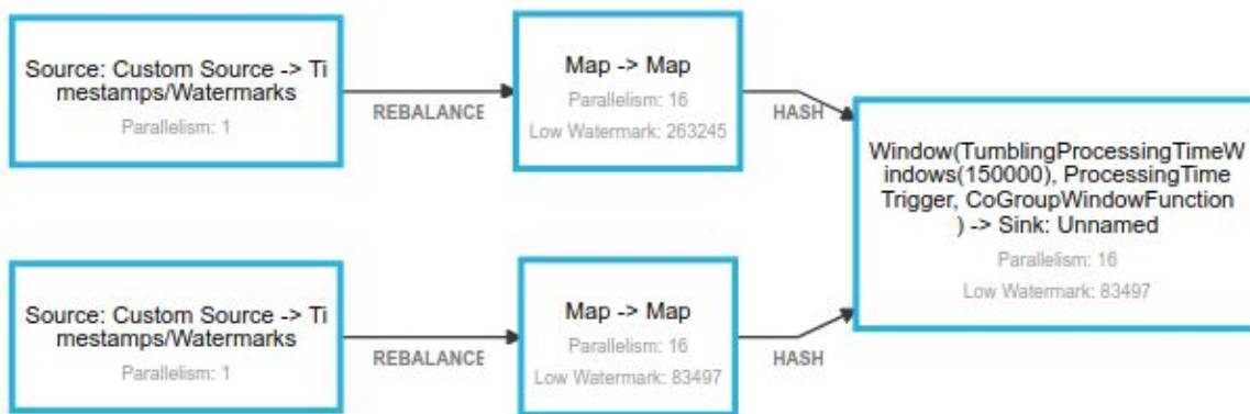
Fig. 53: Flink Dataflow for window operation
