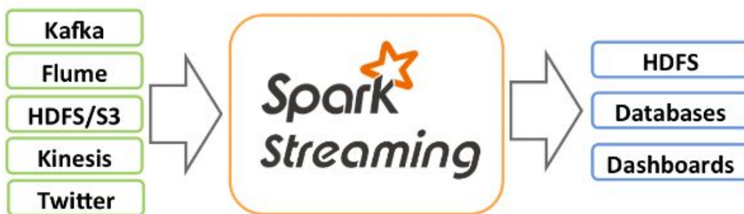
Fig. 8: Spark Streaming architecture
