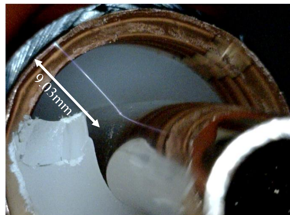
Εικόνα 68: An electric arc (breakdown) in air during DC test
