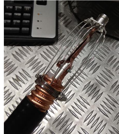
Εικόνα 77: Specially made connector for connecting with the VNA cable
