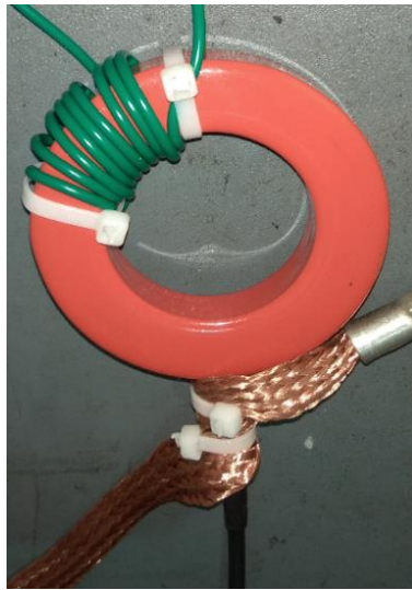
Εικόνα 41: The CT that was used during the experiments
