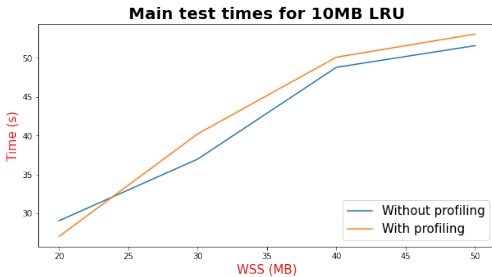
Σχήμα 28: Main test times per WSS, 10MB LRU, 1.000.000 accesses
