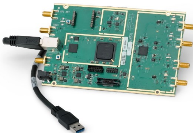
Figure 4-11: The Ettus USRP B210 SDR device used
