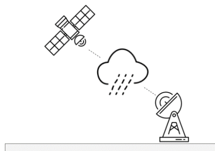
Figure 3-1: A satellite link slant path impaired by atmospheric effects
