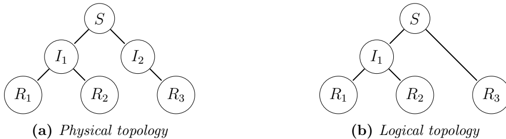
Figure 2.3: Physical (a) and logical (b) topology of the simple-structured network of Figure 2.2 . There is no branching in node I_2 , so it is not visible in logical topology.
