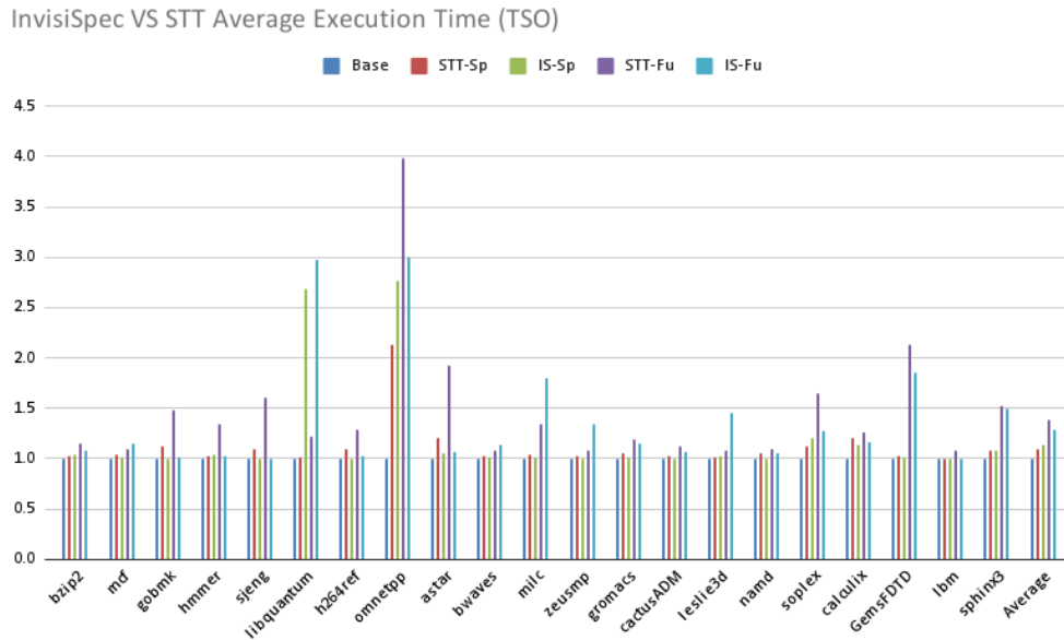
Figure 19: InvisiSpec VS STT average execution time on SPEC2006.
