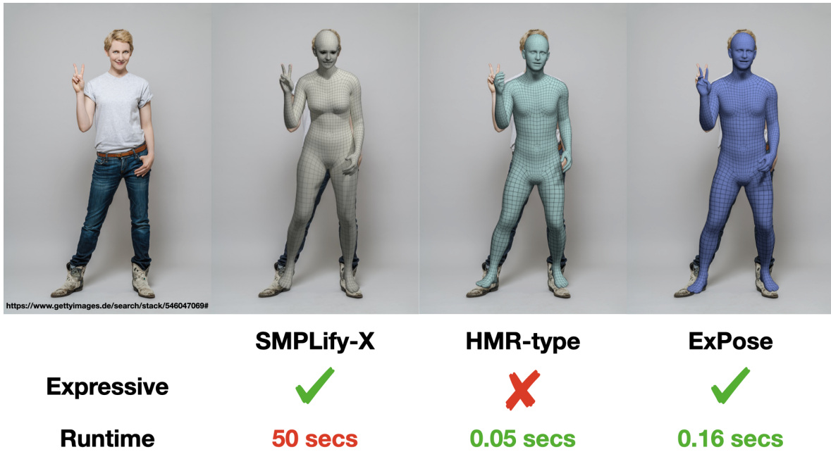
Figure 4.3: Comparison between three state-of-the-art 3D Reconstruction methods for body, face and hands, namely HMR, SMPLify-X and ExPose.
