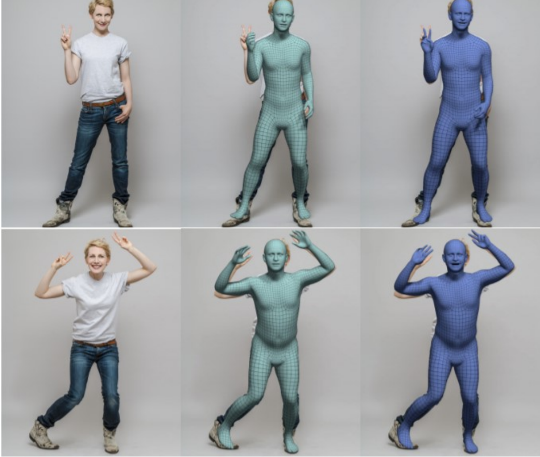
Figure 2.13: Qualitative results of the ExPose method. The raw RGB image is shown on the left. The naive regression from a single body image is shown in the middle, which fails to capture detailed finger articulation and facial expressions. The ExPose results are shown at the right. Note that due to the attention mechanism, ExPose is able to recover details and produce results of similar quality as SMPLify-X, while being 200 times faster. Image from [15].
