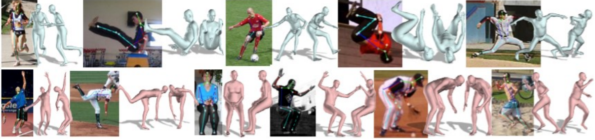
Figure 2.7: Each sub-image shows the original image with the 2D joints fit by the CNN. To the right of that is the estimated 3D pose and shape and the model seen from another view. Image from [7].
