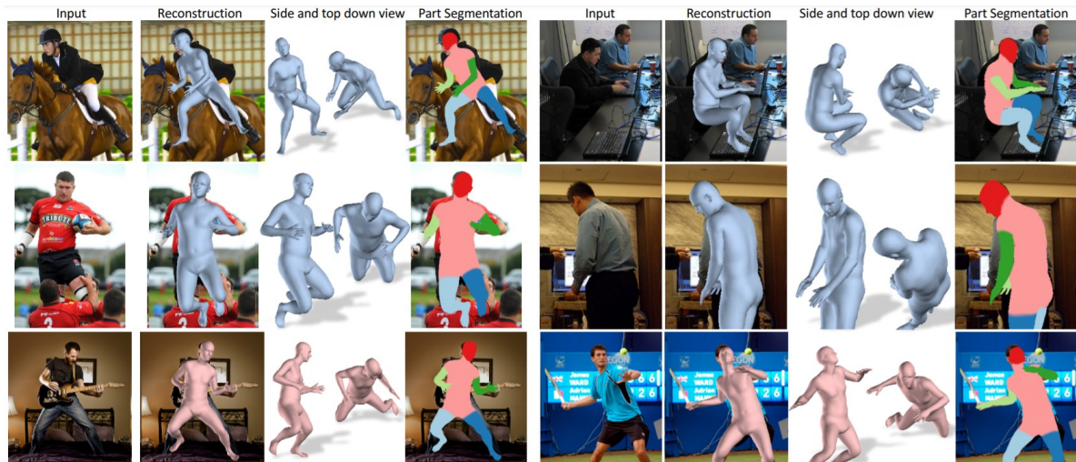
Figure 2.9: Human Mesh Recovery (HMR) qualitative results using end-to-end adversarial learning of human pose and shape. The first two rows show results from the HMR model trained with some 2D-to-3D supervision, while the bottom row shows results from a model that is trained in a fully weakly-supervised manner without using any paired 2D-to-3D supervision. The full 3D body is inferred even in cases of occlusions and truncations. Head and limb orientations are captured as well. Image from [34].
