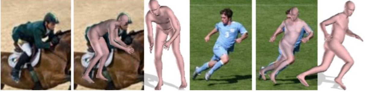
Figure 2.5: Two examples from the 3D pose and shape estimation using the SMPL-ify method. The original image is shown at the left, the fitted model at the middle and the 3D model rendered from a different viewpoint is shown at the right of the figure. Image from [7].
