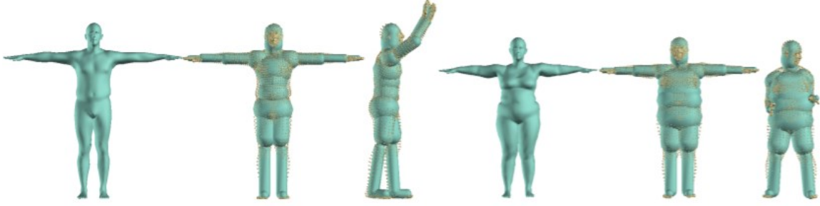
Figure 2.6: Body shape approximation using capsules for two subjects. The original shape is shown at the left, the approximated shape with capsules is shown at the middle, while the capsules reposed are shown at the right. Yellow point clouds represent actual vertices of the model that is approximated. Image from [7].
