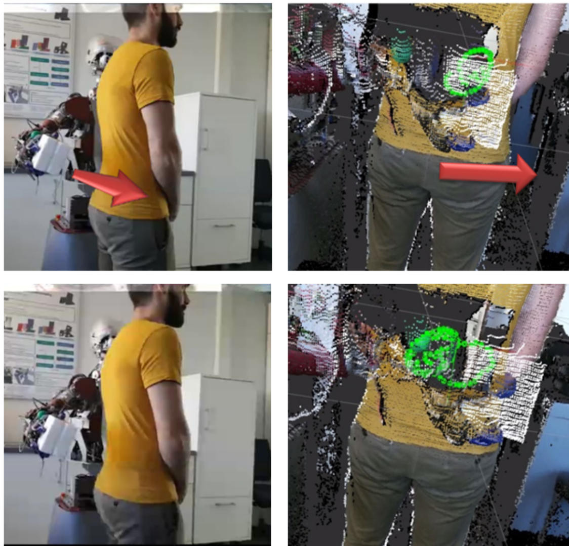
Figure 5.18: Scenario III: ARMAR-III is wiping a male subject's back region. The subject is moving to the right and the robot follows the motion. Left: Side camera view of the subject performing a translation to the right. Right: Zoomed Point cloud view of the experiment highlighting the adaptation of the wiping motion (green trajectory) to the movement of the subject. Safe distance is kept between the back and ARMAR-III's end-effector.
