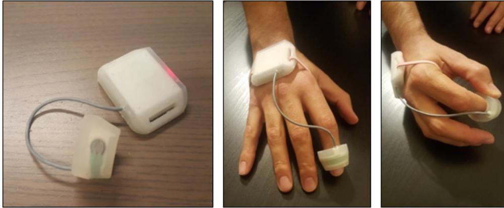
Figure 5.6: a) Motion tracking hand-wearable device. b) Thimble with the embedded pressure sensor for activation).
