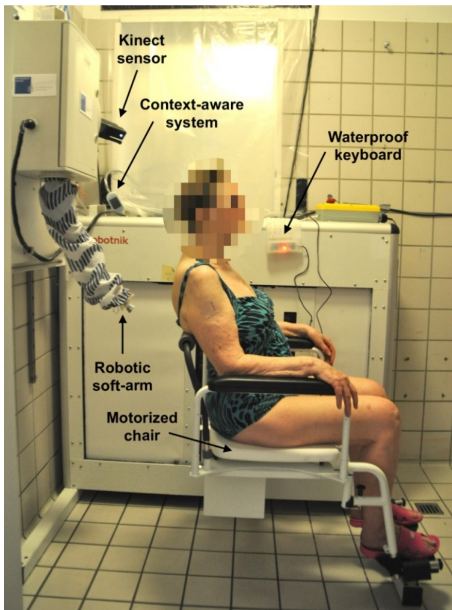
Figure 5.7: Water pouring clinical validation study with the I-SUPPORT bathing robot installed in a typical bathroom of a rehabilitation clinic at a geriatric hospital.
