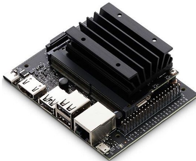
Figure 6.3: Jetson Nano Developer Kit
