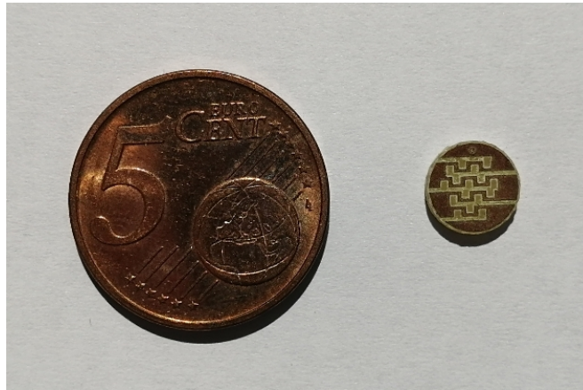
Figure 1.22 Upper patch of the proposed implantable antenna.
