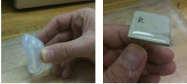
Figure 1.3 Silicone and the antenna encased in the silicone [18].
