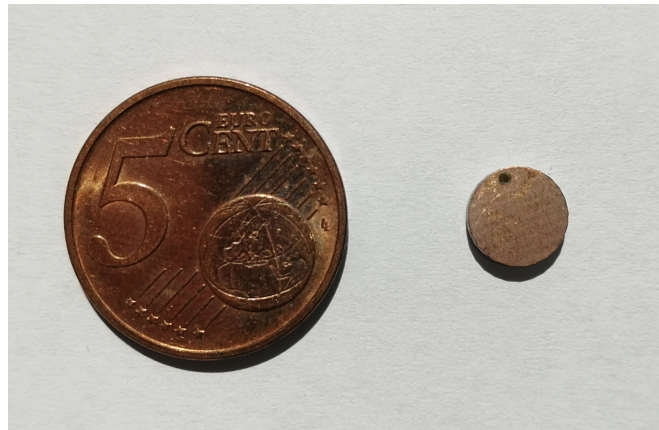
Figure 1.20 Ground plane of the proposed implantable antenna.
