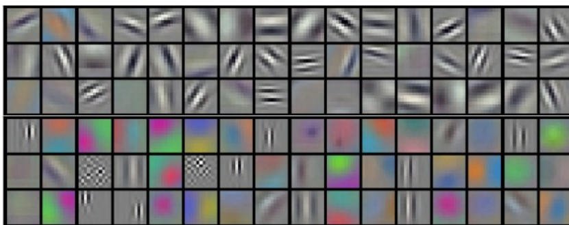
Figure 2.4. 96 filters learned by the first convolutional layer of AlexNet. Source: [4]
