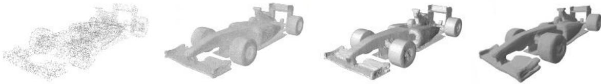
Figure 4.10: Renderings by [18]. Left to right: input point cloud, point cloud sampled with Newton-Raphson method, mesh reconstructed from samples point cloud with ball-pivoting and rendering with sphere tracing. Figure adapted from [18].
