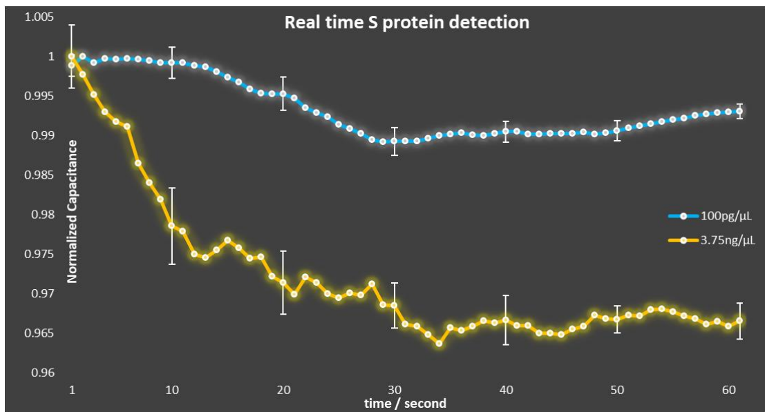
Figure 37. Normalized capacitance change over time due to the binding of S protein.
