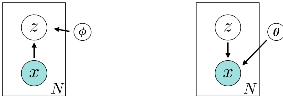
Figure 6.1: Directed graphical models for (a) the approximate posterior q_\phi(\mathbf{z}|\mathbf{x}) and (b) the probabilistic decoder p_\theta(\mathbf{x}|\mathbf{z}) . The coloured node indicates the observable random variable and the nodes outside the box are model parameters.
