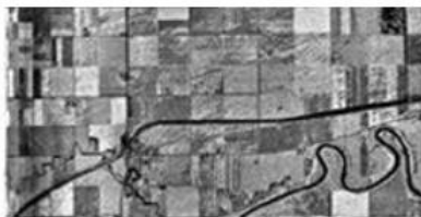
Slant-Range Scale Distortion
