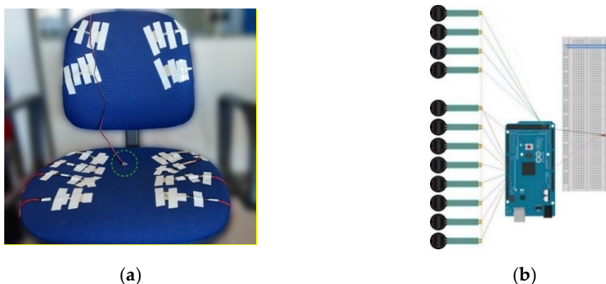
Figure 4-6: (a) Smart chair with initial arrangement of 12 pressure sensors. PulseSensor (placed in the user's ear lobe) is marked by the green circle.; (b) Microcontroller setup for acquisition of data from the smart chair.
