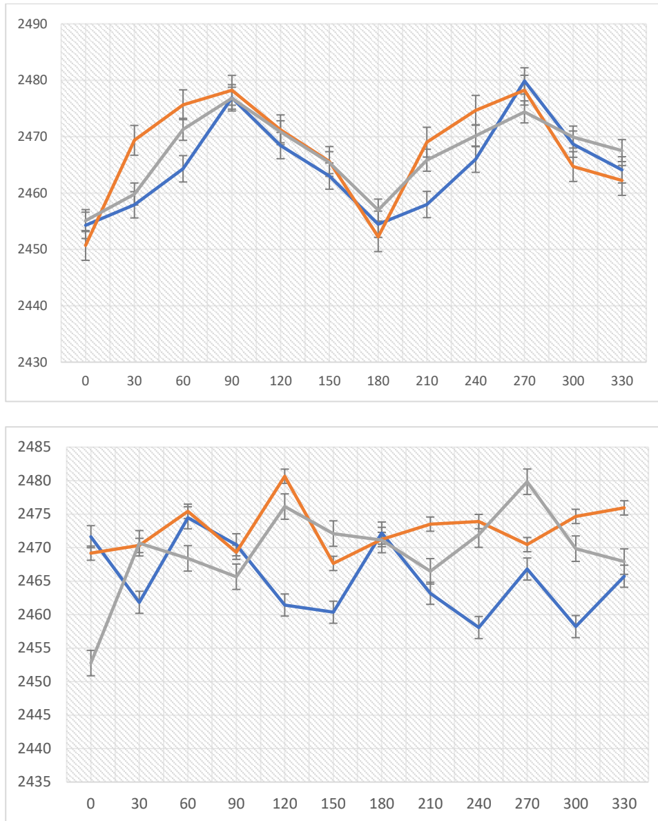
Figure 38. Experimental measurements for flawless SU-T (above) and with added defect (below), ( S_1 -blue, S_2 -orange, S_3 -gray).
