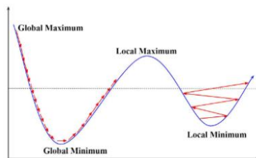
Figure 3: A Demonstration of the Difference between the Local and Global Maximum and Minimum Values and the Learning Rate (shown in red) that Determines the Magnitude of the Updates to Model's Weights. Image Credited to [11].
