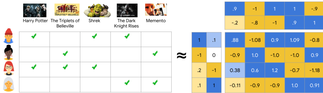
Figure 4.9: A visualization of matrix factorization. The model learns a user embedding matrix and an item embedding matrix such that their product is a good approximation of the user-item interaction matrix. Retrieved from [25].
