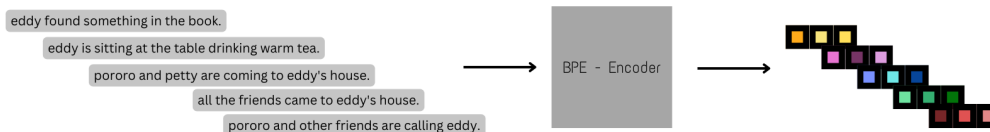
Figure 8.2.1: The sentences of a story are BPE-encoded to obtain text tokens
