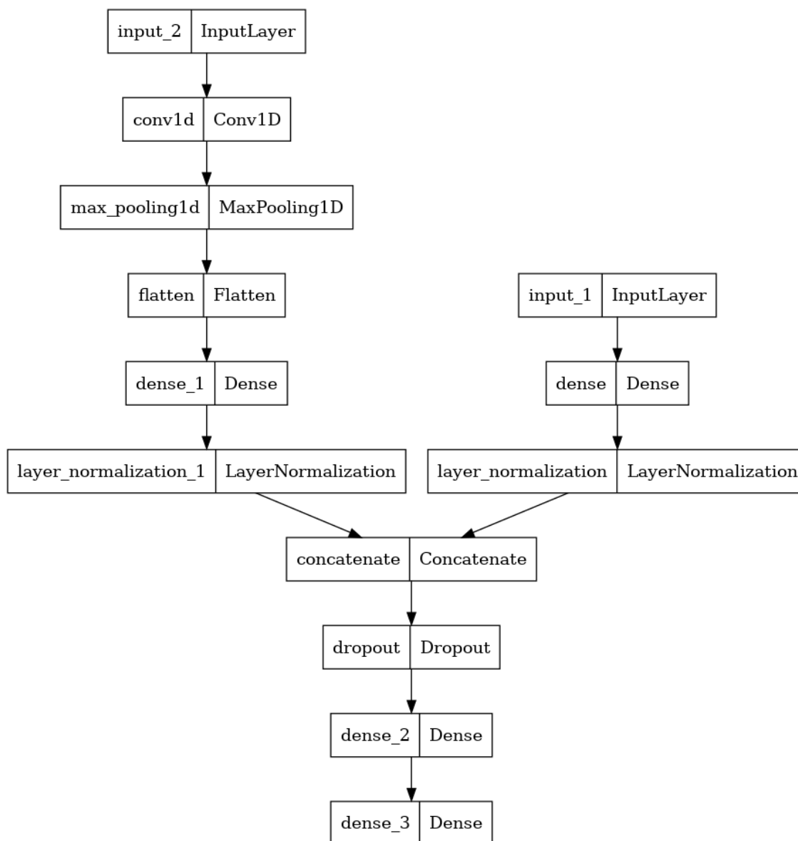
Figure 3.5. Convolutional neural network's structure. input_1 are the embeddings and input_2 are the reuse distances.
