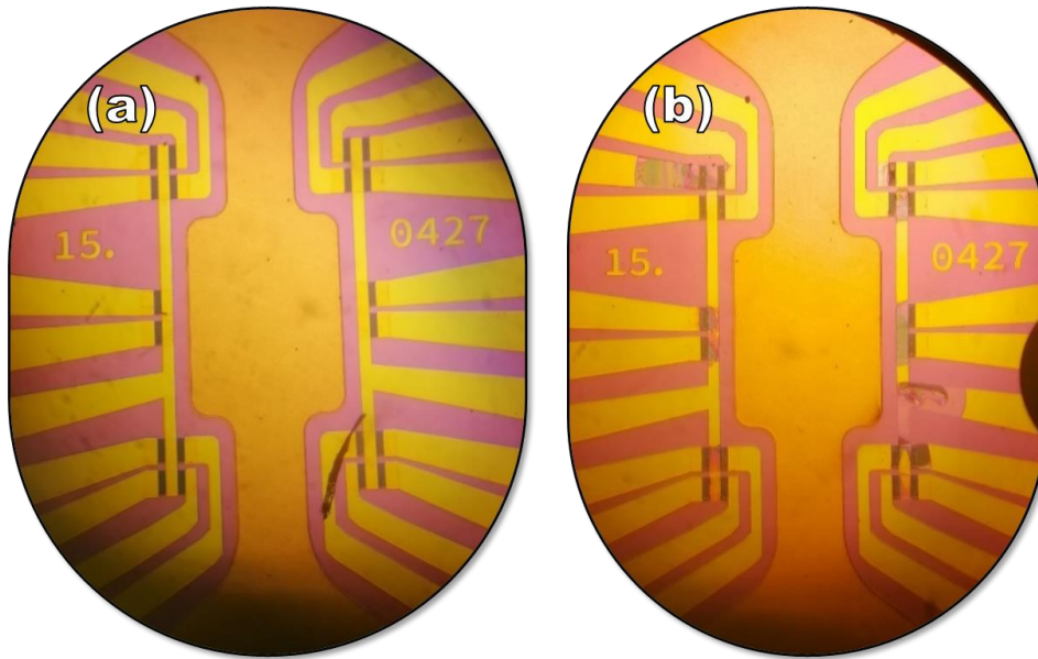
Figure 5.2: Chip 150427 (a) before sampling measurements and (b) after sampling measurements, where the electrochemical etching is obvious in many spots.
