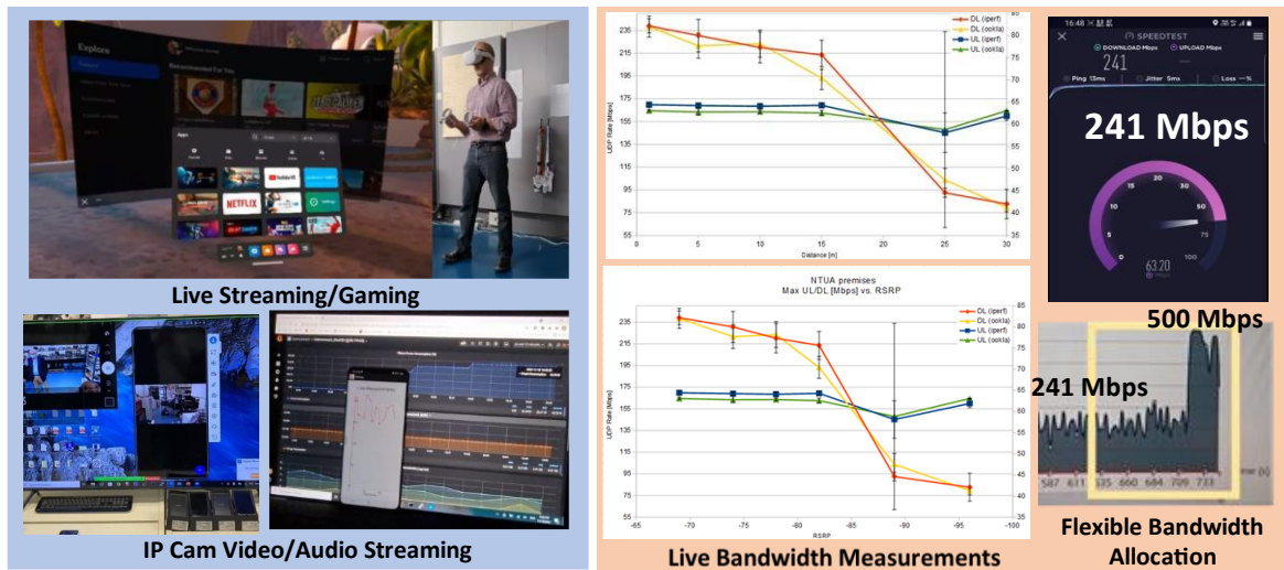
Figure 60. Service/Control layer evaluation of analog TxRx interface, including: Dynamic capacity reconfiguration, Live latency/bandwidth measurements, Live Bandwidth measurements, and Demonstration of the uninterrupted operation of AR/VR gaming, 4K video streaming, and IP videos, over the presented deployment.
