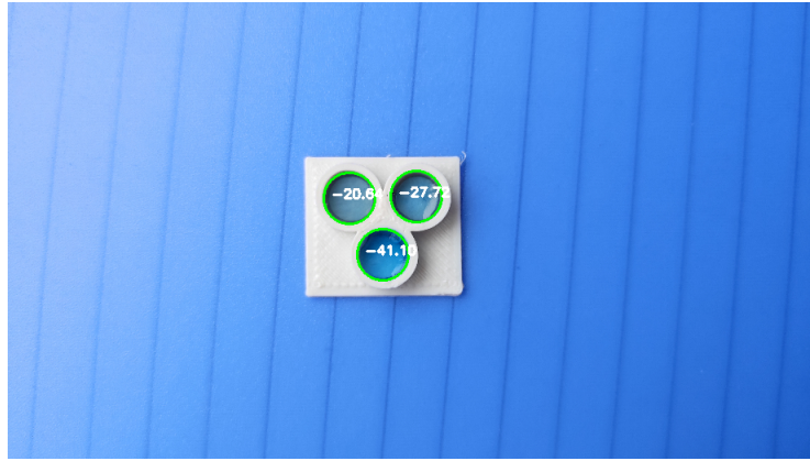
Figure A.2.6. Color assessment for each well by b^* channel.
