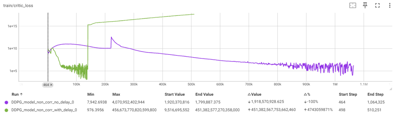
Figure 66 : Comparison of Critic Loss (Log Scale) per Timestep of DDPG Non-Corrective With Delay and No Delay Models
