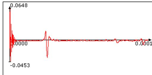
**Figure 8.38.** A typical pulsed voltage output of the search coils of Figures 8.36 and 8.37. The time scale (X-axis) is in seconds and the voltage scale is in Volts.
